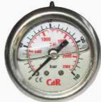
CDR.75S401N1P Professional pressure gauge with rear entry, case and ring made of AISI 304 stainless steel, temperature -20°C (-40°F) -80°C (-170°F). Scale: bar (black), psi (red). WARNING !! To avoid damaging pressure gauges, we recommend using pressure gauges with a full scale range of twice the working pressure of the pump.
