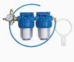
ZX.0696-7-R Water inlet kit 7", complete with pressure stabilizer, support bracket, string-wound cartridge of 1micr polyphosphate anti-limescale container and filter tightening spanner
