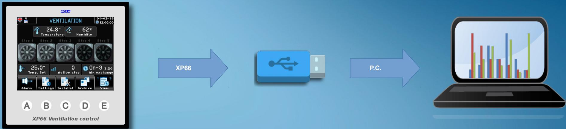
The communication with the outside world is performed by USB key.
