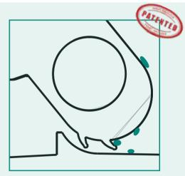
The air inlet uses the venturi effect to draw in the air inside the house along with the incoming air. The round opening keeps the air in the house moving to prevent condensate from forming on the valve.
